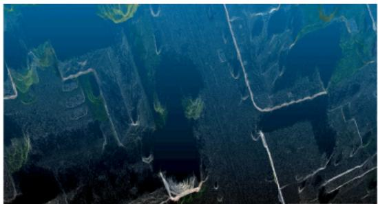
Walls are visible as dense lines in photogrammetric or laser scanning point clouds.
