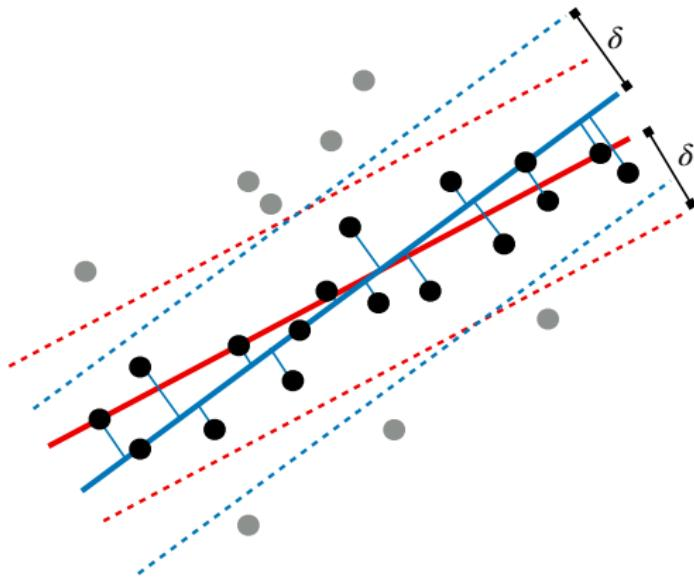
Using a Principal Component Analysis, the plane model can be optimized such that distances between plane and inliers become minimal subject to keeping the direction of the normal in the projection to the ground plane.
