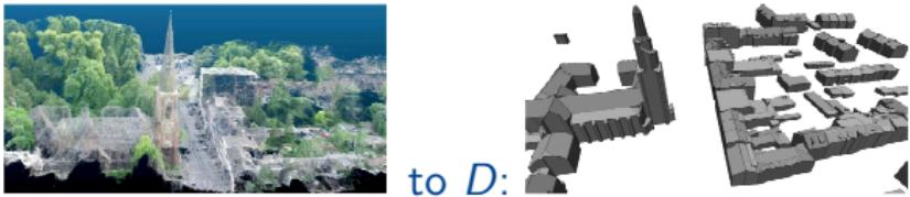
**procedure** ICP(point cloud  $S$ , city model  $D$ , convergence criteria)
