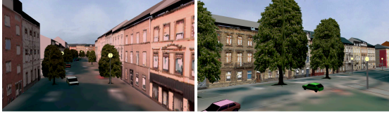
Figure 11: Texturing of facades requires higher precision of z -coordinates. Black areas between textures and roofs indicate that walls are too high whereas slopes of roof facets are too small.
