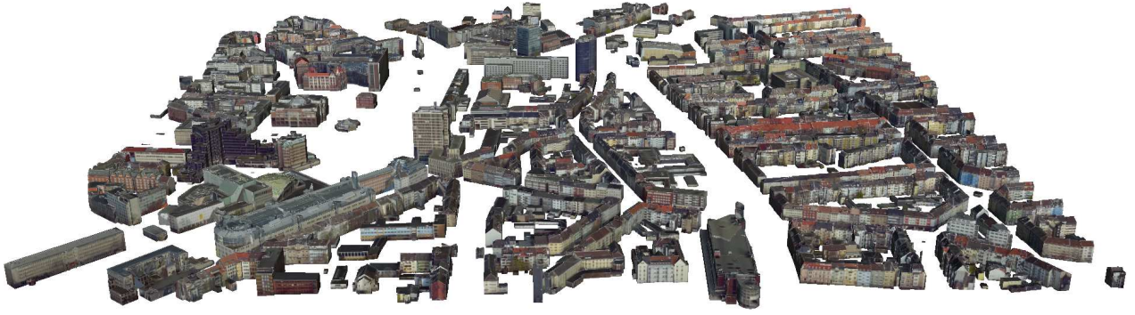
Figure 5: Test data: Our variant of RANSAC was used to estimate roof facets of this model of a square kilometer of the city of Dortmund
