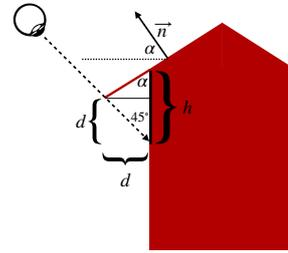
Figure 8: Estimating the size  $d$  of an overhang with normal  $\vec{n}$  from a texture in which the roof section has height  $h$ , see (7).
