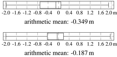
Figure 13: Quality of overhang sizes estimated from sparse airborne laser scanning point clouds: The box plots show the distribution of differences between  $\sigma$  and  $\gamma$  (see Section 5.2) for the same two square kilometers as in Figure 10.
