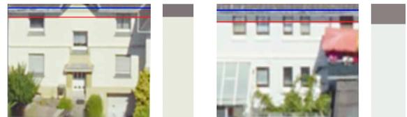
Figure 12: The blue lines separate the roof and facade based on an edge image, the red lines separate the dominant colors of the roof and facade.
