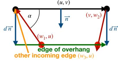
Figure 2: An orthogonal attachment of an overhang to the edge  $(u, v)$  might intersect with walls belonging to incoming edge  $(w_1, u)$  and outgoing edge  $(v, w_2)$ . In that case, the red vertices have to be used in the construction of the overhang.
