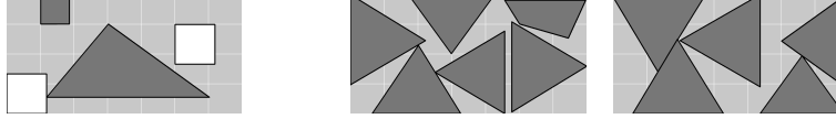
Fig. 1. The distance condition (2, 3) requires that each square of the background grid has to be at least partially covered. Left: A feasible one-bin layout for two tiles (grey) with two support plates (white). Right: An optimal solution using two bins without support plates (instance 3 in Table 1).
