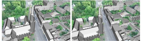
Figure 8: A city model is drawn onto a video frame using the frame's SfM camera transformation and estimated camera parameters. The upper picture is based on a coarse manual alignment between SfM point cloud and UTM coordinate system. The second picture shows optimized alignment.
