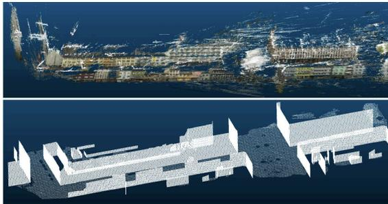
Figure 1: SfM point cloud, and cloud sampled from CityGML walls and merged with terrain points from airborne laserscanning
