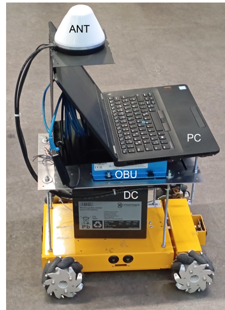
Fig. 4. Equipped vehicle for measurements in cellar.
