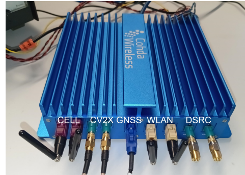
Fig. 3. Cohda Wireless OBU MK6 with connections.
