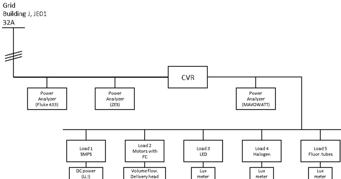
**Figure 1:** Experimental setup of the CVR unit, the loads and measurement equipment in the laboratory
