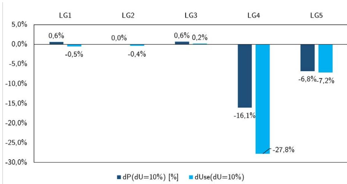
**Figure 4:** Change in power consumption and useful work of the load groups 1 to 5 for a voltage reduction of 10 %
