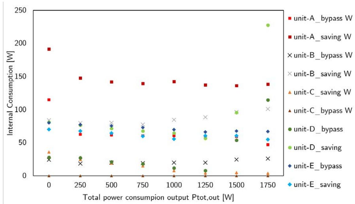
**Figure 3:** Internal consumption for CVR units A, B, C, D and E in bypass and saving mode with increasing total power consumption  $P_{tot,out}$
